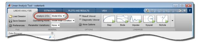
**4** Linearize the model with the specified I/Os, and generate a Bode plot of the linearized model.
